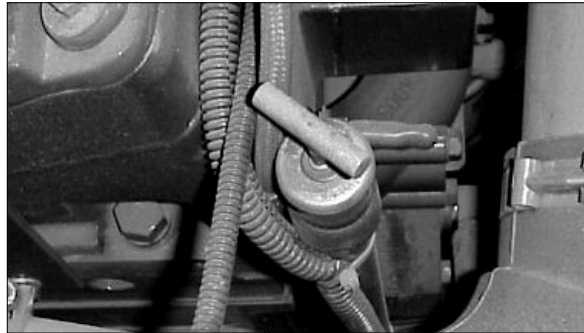
Transmission Oil Level Dipstick.
